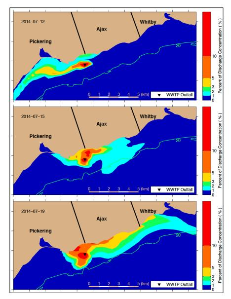
**Figure 9.** Simulated conservative tracer concentration, averaged over the water column and over the day and expressed as a percentage of the discharge concentration. Results illustrate variation in the Duffin Creek WWTP plume for three dates in 2014. The green line is the 20-m depth representing the approximate lakeward extent of colonization by *Cladophora* and taken as the separation of nearshore and offshore waters. Model results are from run#2.
