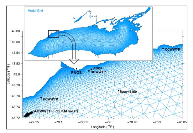
**Figure 3.** Model mesh for Lake Ontario with additional detail presented for the immediate study area. The locations of wastewater treatment plant (WWTP) outfalls, the acoustic Doppler current profiler (ADCP), the Pickering Nuclear Generating Station (PNGS) and the NDBC buoy are identified.
