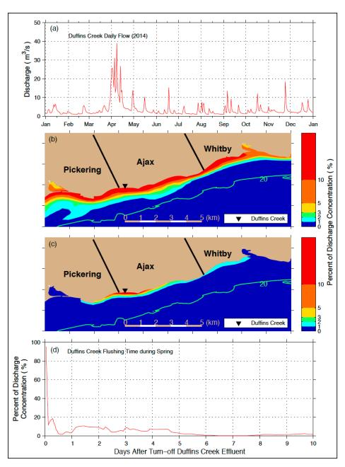
**Figure 10.** Model inputs and results for tributary simulations: (**a**) Duffin Creek flows for 2014, (**b**) Duffin Creek plume for high-flow conditions, 4–10 April 2014 (model results are from run#3), (**c**) Duffin Creek plume for low-flow conditions, 13–19 July 2014 (model results are from run#4), and (**d**) purging of the Duffins Creek plume from nearshore waters (model results are from run#5).
