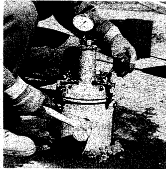
Fig. 16-5. Pressure-type meter for determining air content. (68766)
