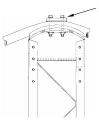
Keep saddle cover plate loose during bridge erection time, but tighten it firmly before removing the temporary side struts at the bottom of the tower.
