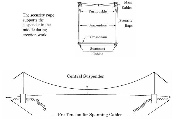
Tighten the spanning cable to some extent; now the cables are ready to be fixed to the suspenders.
