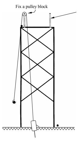
Main Cables at either side of the Tower Temporary device for lifting the main cables (supplied with Top Element)
