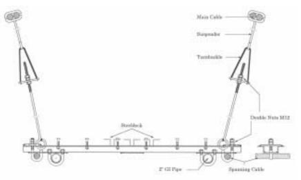
The G.I. pipes have to be fitted before the outer rows of the steel decks are mounted in the following way:
