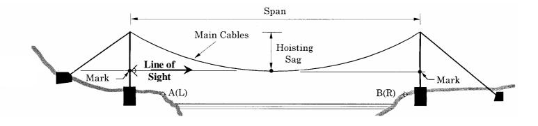
Also check the sags from time to time when the fitting works are going on. Different elongations may take place due to dissimilar hidden cable relaxations when the tension increases. Adjust possible sag differences with the help of the turnbuckles at the main cable anchor so that the Main Cables are always parallel and compare the dead load sag with the pre-calculated values.
