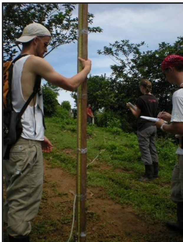
Image 4: Surveying using a water level. Photo by Ashley Thode.
