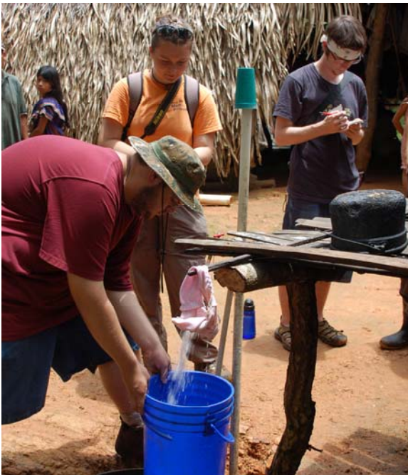
Figure 14: Flow rates being measured with a stopwatch and 5 gallon bucket.
