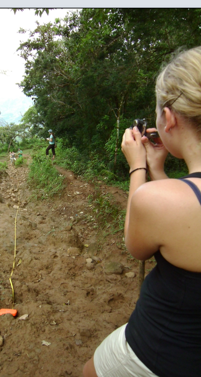
Above: Collecting survey data in the community with an Abney Level. Photo taken by Angella Mickowski Right: Location of water source. Photo taken by Rebecca Bender
