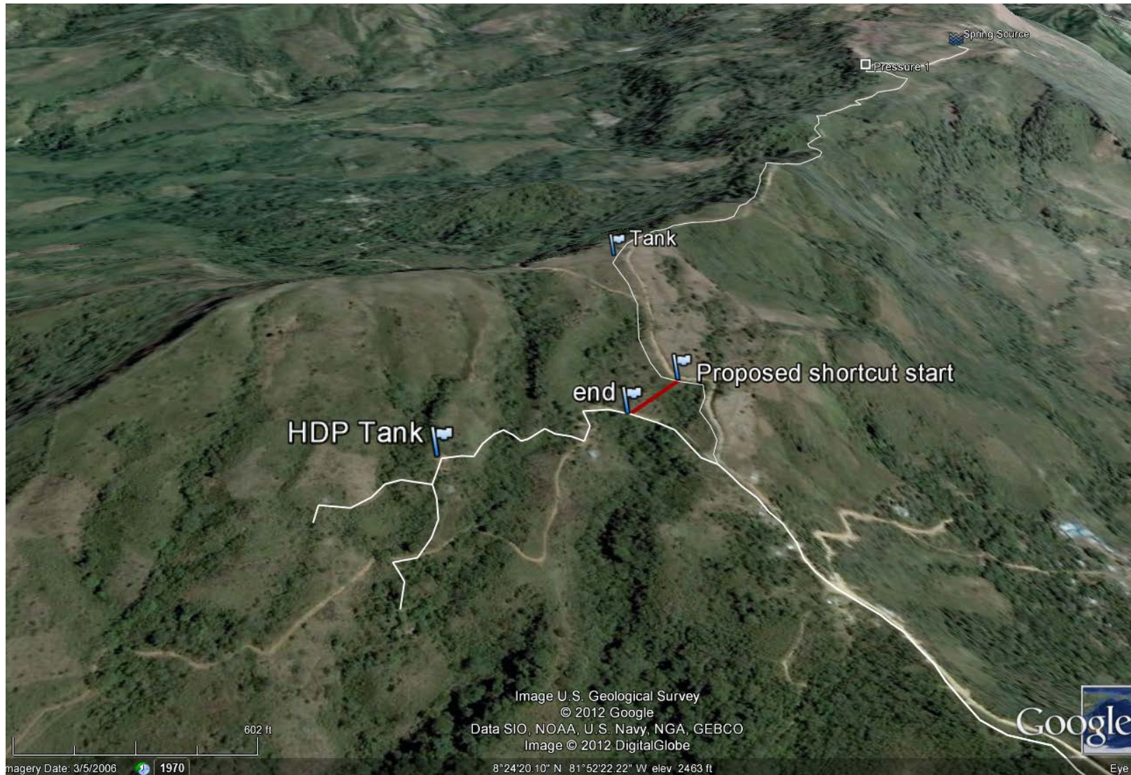
Figure 12 Courtesy of Google Earth Pro. Topographical layout of the suggested shortcut to Cerro Peña in order to provide adequate supply, and reduce piping cost.
