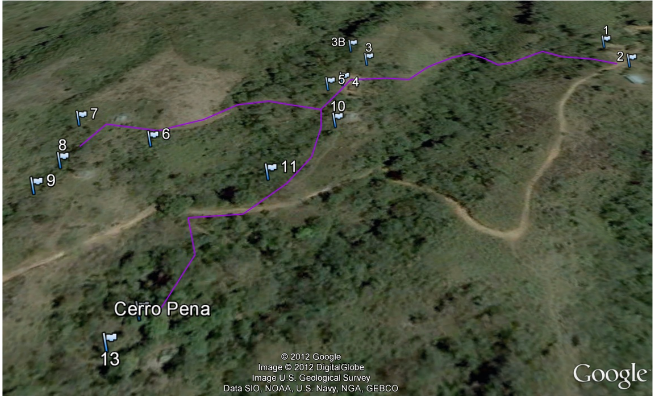
Figure 2. The spigots in Cerro Peña along the main distribution line. Note: no branches off main distribution are shown
