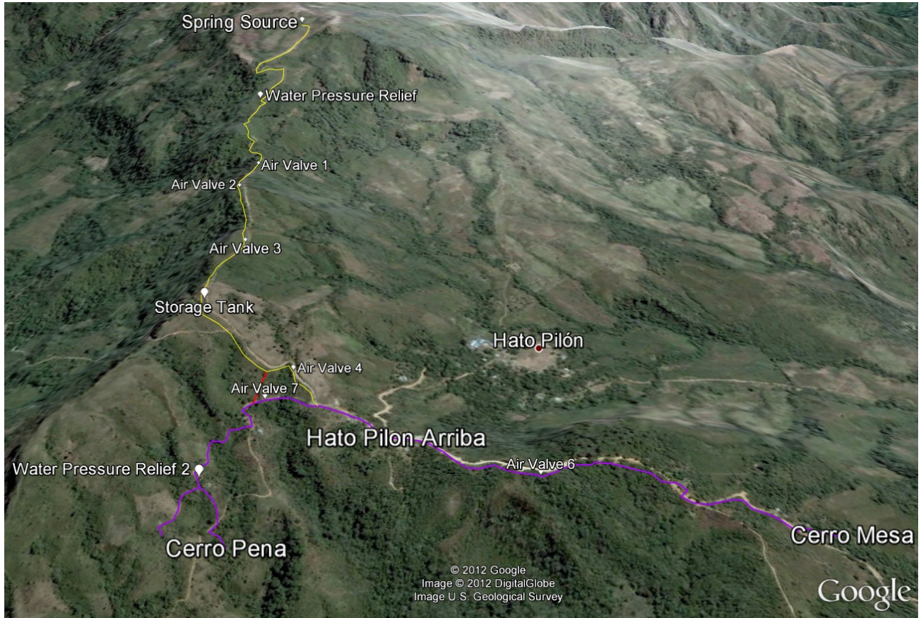
Figure 5. Suggested locations of recommended pressure relief basins, storage tank, and air relief valves
