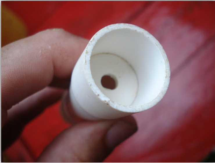
Figure 19. Example of flow reducer that would be placed on the system. These attachments can be handmade by melting PVC pipe, and may be placed on every 1/2" branch of the system.
