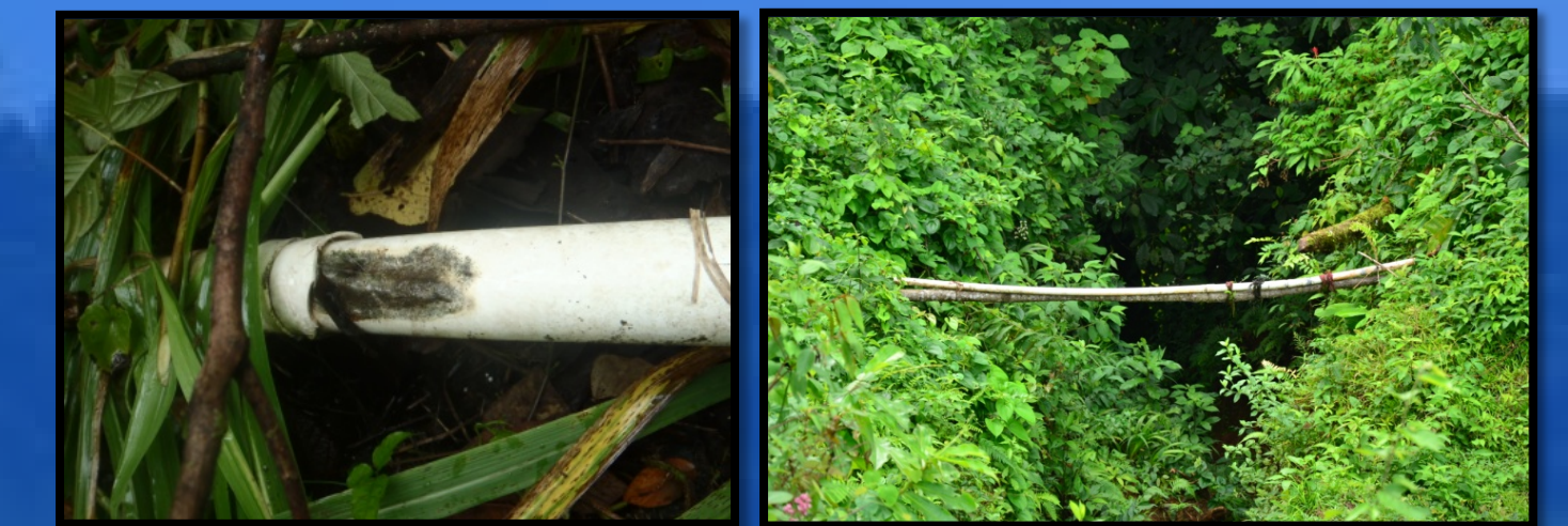
Figure 12 (top left): PVC damage from UV exposure
