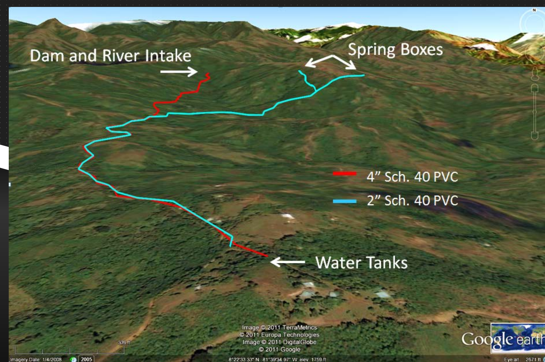
Pipeline routes to storage tanks
