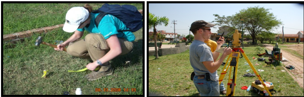
Figure 8: Kim Marking a Control Point; Aaron Surveying the Soccer Field
