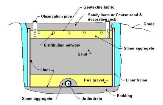
Figure 17: Single Pass Sand Filter Bed (WI Dept. of Commerce, Doc. SBD-10595-P)
