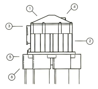
**1. Valve Top:** A high strength metal die cast top which is secured to the valve body by eight stainless steel screws.
