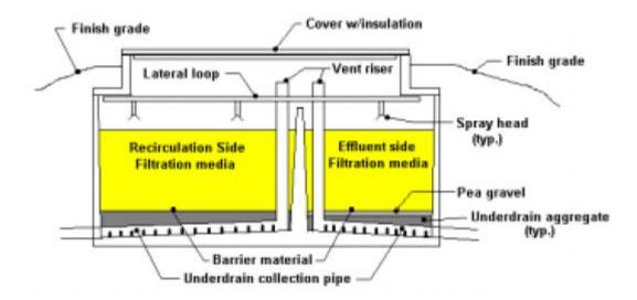
Figure 18: Split Bed Recirculating Sand Filter (WI. Dept. of Commerce, Doc. SBD-10656-P)
