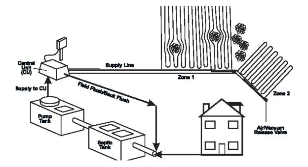
Figure 19: Drip Line Effluent Dispersal System (EPA Doc. EPA 625/R-00/008)
