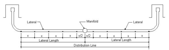
Figure 3 – Number of Orifices in a Distribution Line
