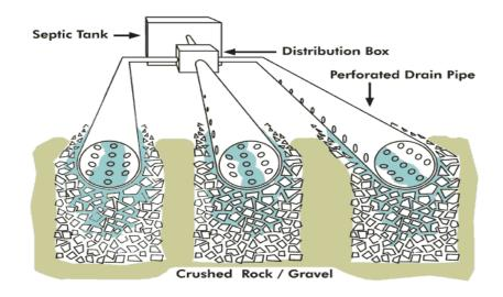
Figure 22: Gravity Drainfield
