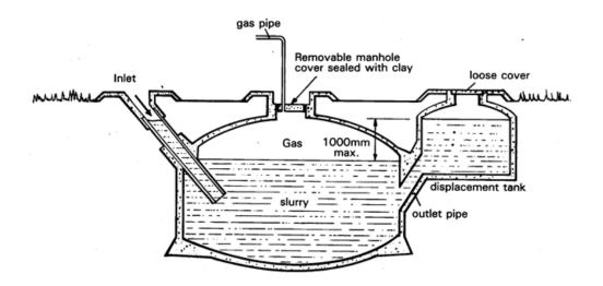
Figure 21: Fixed Dome Biogas Digester (FAO Irrigation and Drainage Paper 43)
