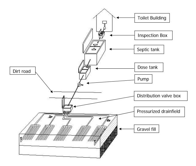
Figure 23: Perspective drawing of proposed septic system design for CLE
