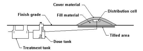
Figure 20: Mound Effluent Dispersion System (WI Dept. of Commerce, doc. SBD-10691-P)
