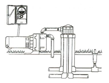
For direct pump - fed installations, the HYDROTEK® 6000 Series Valve is directly connected to the discharge side of the pump and is cycled from one zone to the next by turning the pump off and on . Install the valve as close to the pump as possible and ensure suction line to the pump has a proper check valve installed and all joints are completely sealed.
