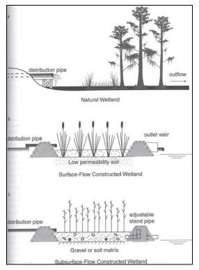
Figure 11: Types of wetland treatment systems (top to bottom): Natural wetland, Surface-flow constructed wetland, and Subsurface-flow constructed wetland
