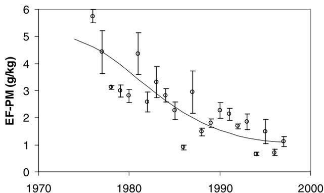
**Figure 5.** Diesel emission factors from *Yanowitz et al.* [2000]. Not shown is a single high test from a 1974 vehicle. Error bars are standard deviation of dynamometer tests divided by  $\sqrt{N}$ . Dashed curve represents best fit.
