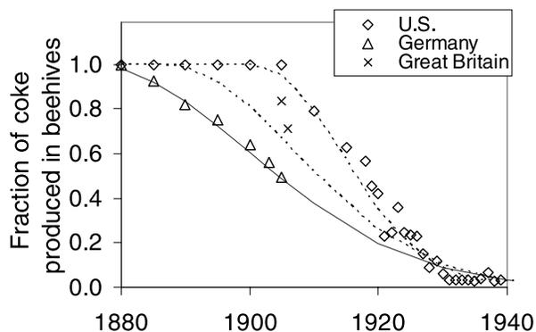
Figure 4. Fraction of coke produced in beehives.
