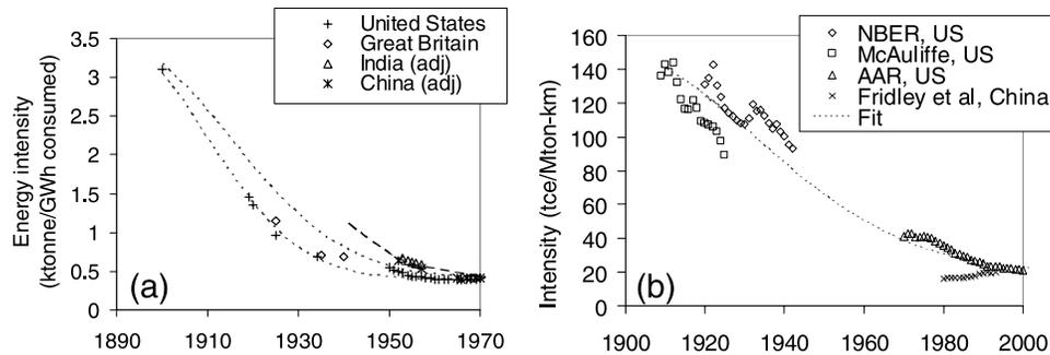
**Figure 2.** Energy intensity for (a) coal-fired electrical power plants and (b) rail freight. For power plants, the short-dashed lines show  $s = 20$  and  $s = 25$ ; we use  $s = 22$ . Intensities for India and China are corrected to heat content of 26 MJ/kg. For rail freight, data before 1940 and China data are coal-fired locomotives; AAR data are mostly diesel locomotives. Abbreviations: NBER, National Bureau of Economic Research; AAR, Association of American Railroads.
