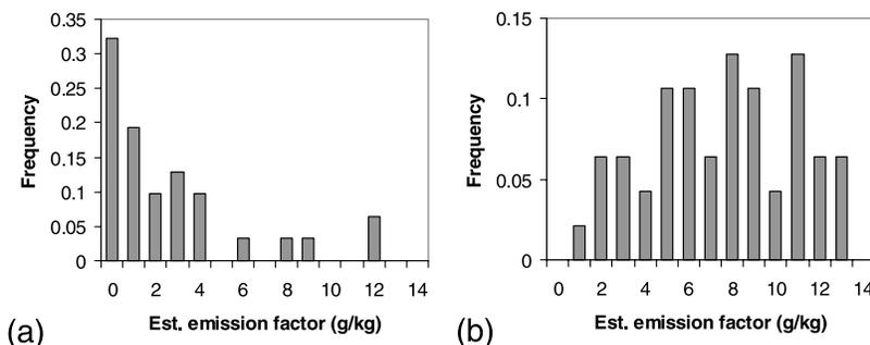
**Figure 3.** Total particulate matter emission factors for (a) chain-grate and (b) hand-fired stokers, derived from opacity and operation data as discussed in section 4.1. For chain-grate stokers, *N* = 36, and for hand-fired stokers, *N* = 61.
